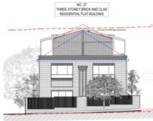
Figure B: Street elevational denoting the extent of the breach above the maximum 9.5m height line viewed from the Boundary Street frontage (Source: Alchemy Architecture, 28.3.2023 – RO4)
