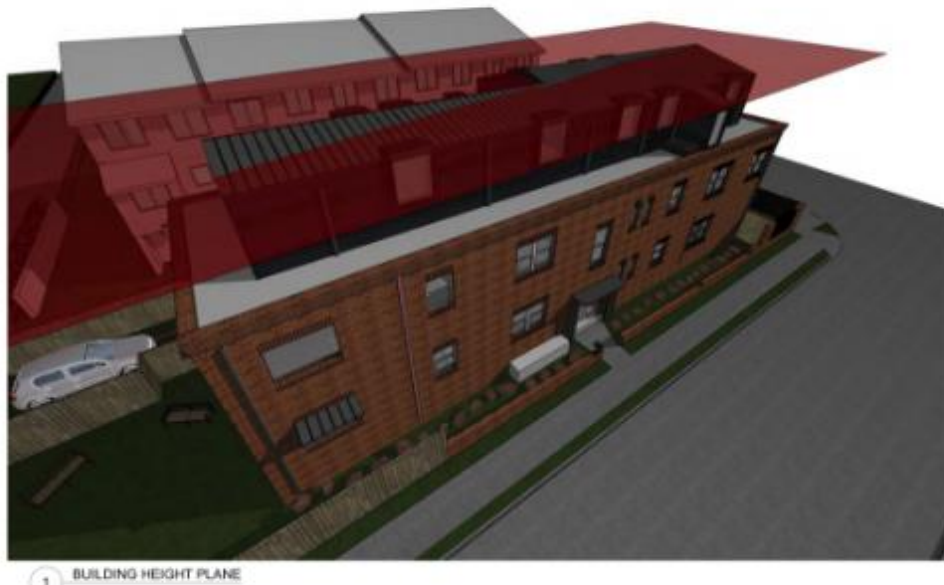
Figure C: Height plane diagrams demonstrating the area of the roof ridge above the 9.5m height limit (Source: Alchemy Architecture, 28.3.2023 – DA20 R04)
