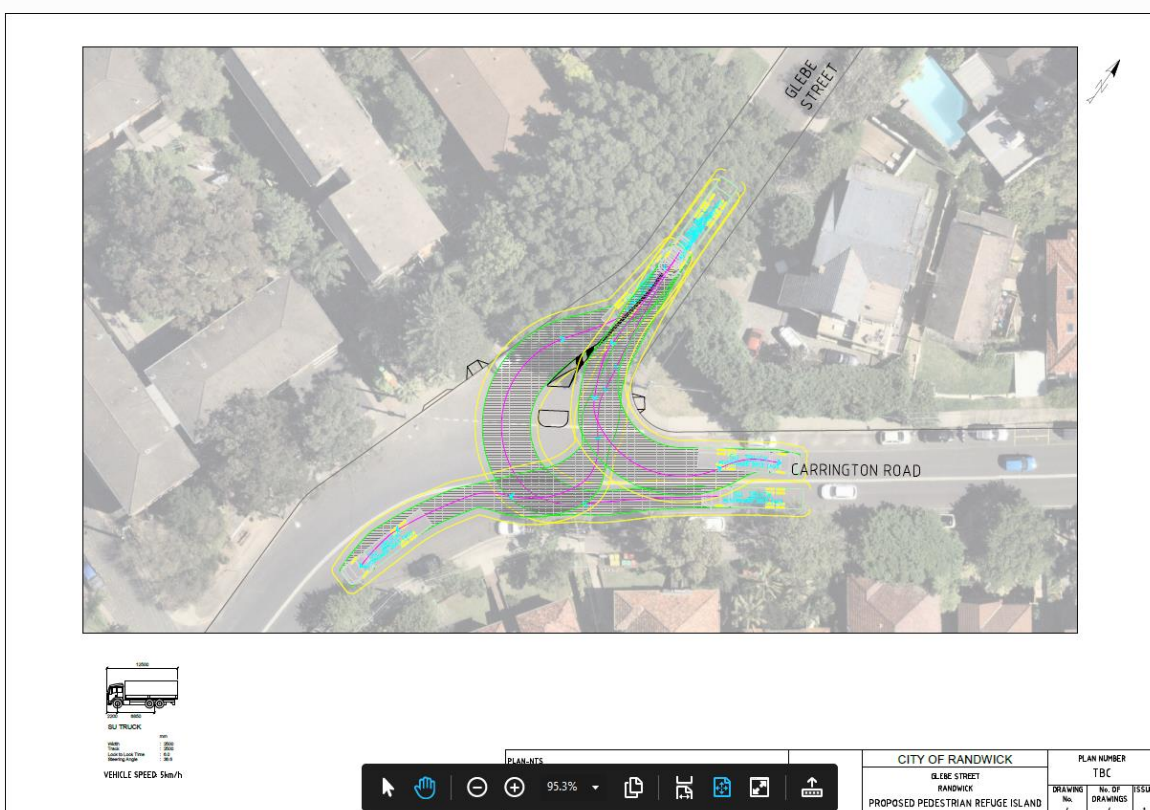
Fig 4: Swept Paths showing Heavy Vehicles (12.8m long)
