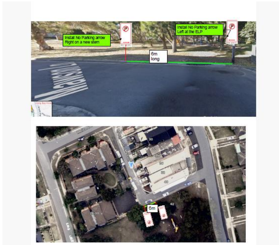
Fig 1: Work instruction for proposed 6m long No Parking section in Mawson Lane, Chifley, SR- 805966
