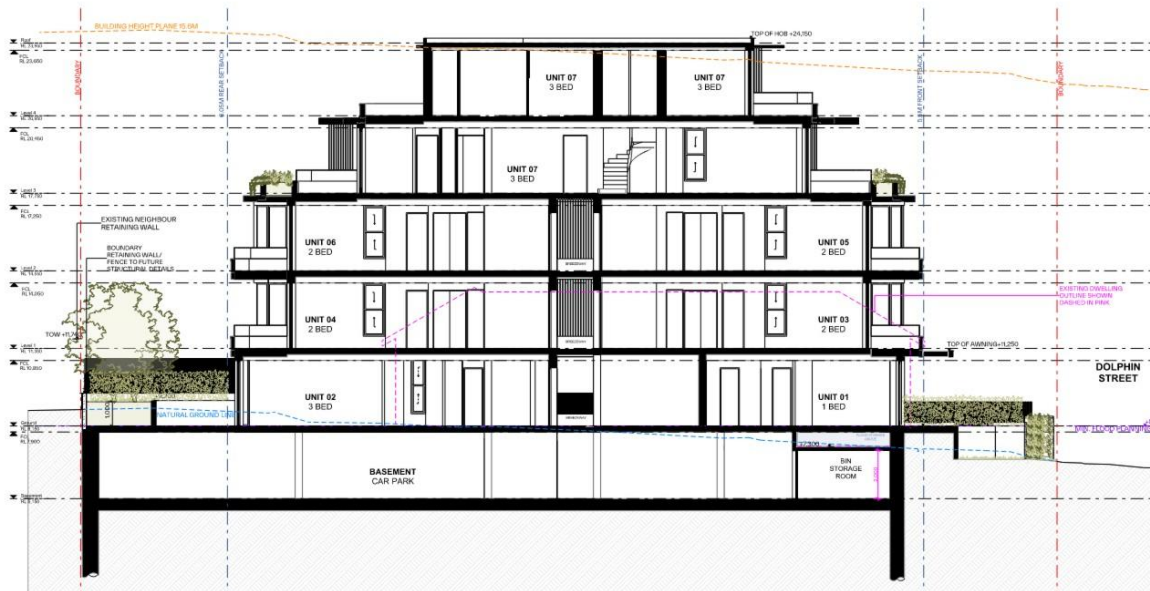
Figure 18: Long section (Source: pbd architects)
