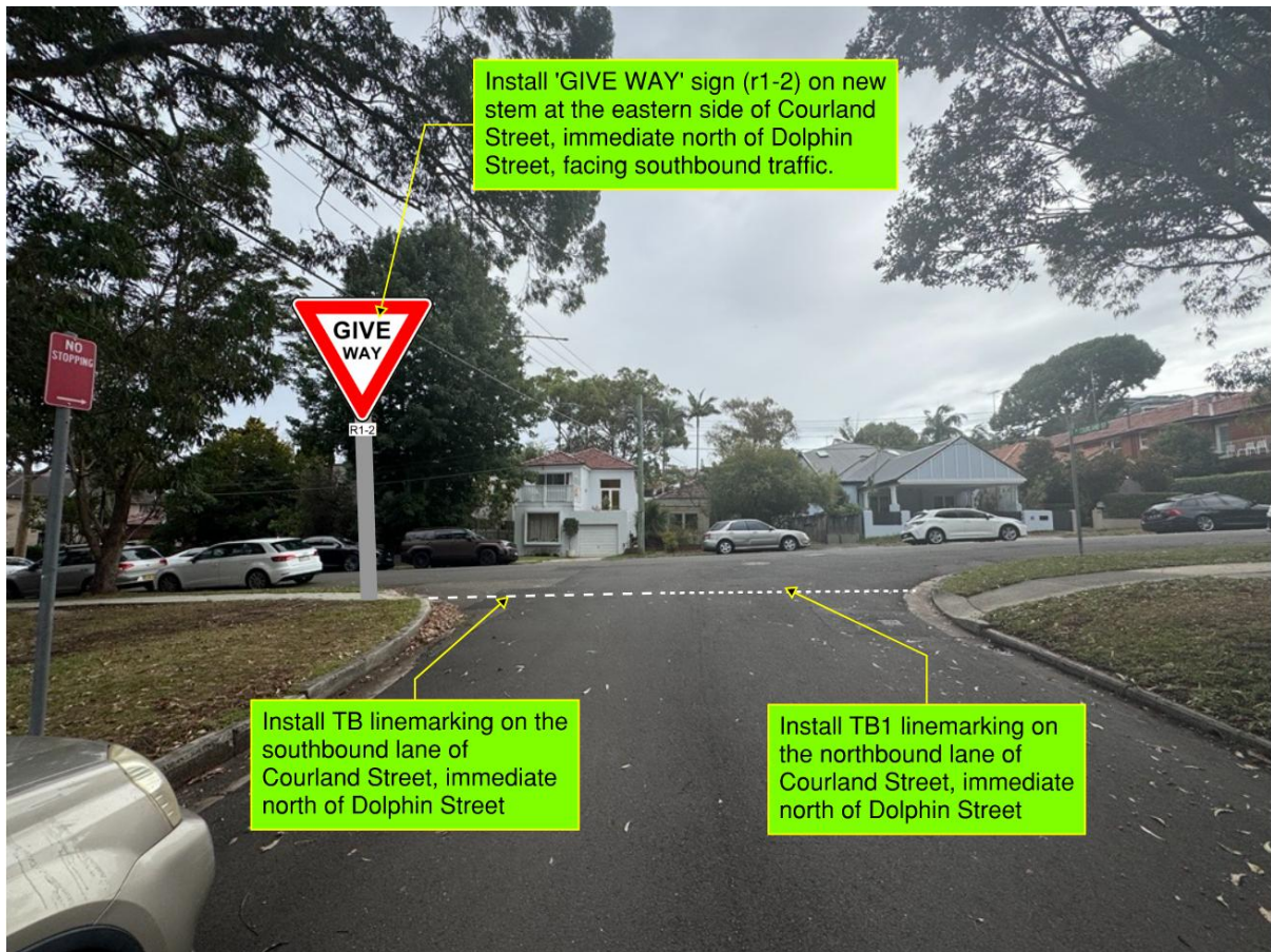
Figure 2: Street View (Signs: SR-791611 and Lines: SR-791612)
