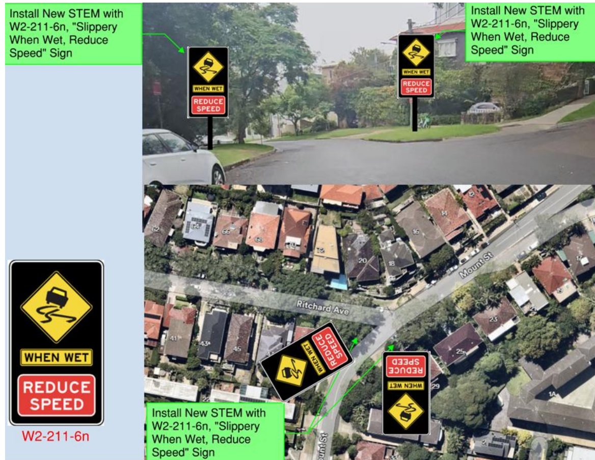
Figure 1 signage to be installed
