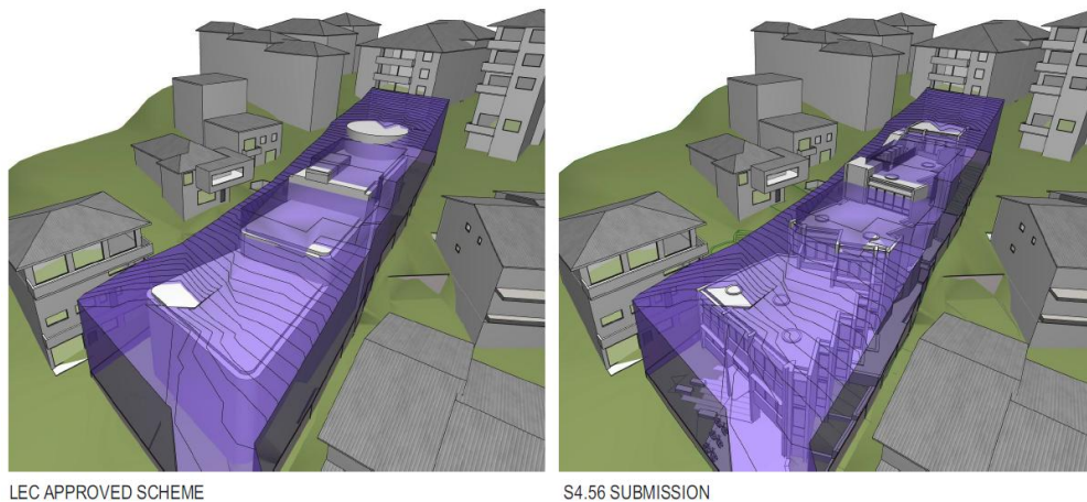
Figure 24: Building height plane diagrams of development consent DA/222/2020 (as conditioned) and proposed in the amended modification application (Source: TonkinZulaikhaGreer)
