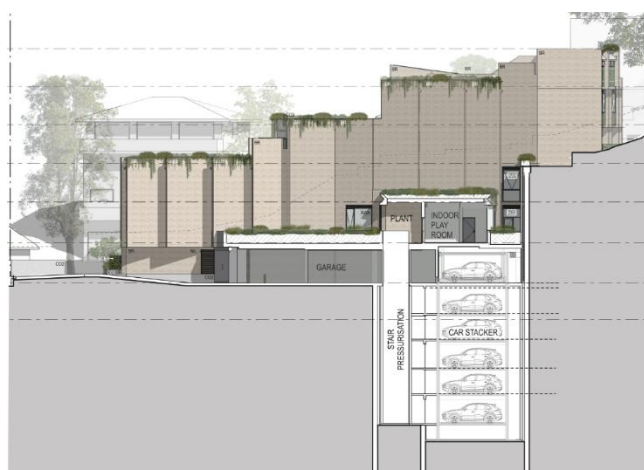
Figure 12: Originally proposed eastern elevation showing the car stacker system (Source: TonkinZulaikhaGreer )
