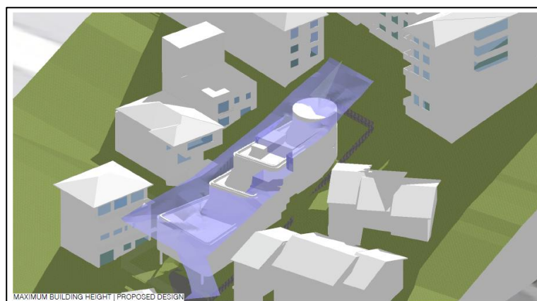
Figure 23: Building height plane diagram of development consent DA/222/2020 ( Source: SHED )
