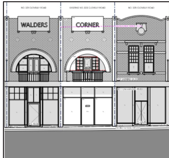
Figure 8: Southern elevation of the proposal, illustrating reinstatement of a first-floor balcony with balustrading configured to match that of No. 321 Clovelly Road.
