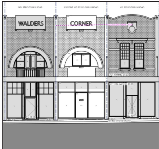
Figure 7: Existing southern elevation of building noting first floor level balcony is enclosed.
