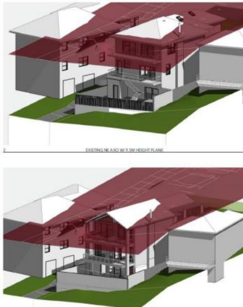
Fig 1: Extract of NE Height Plane Diagram illustrating the extent of the existing and proposed height breach (Source: Richard Coskie)
