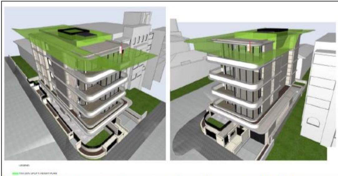
Figure 38: Extract of the height plane diagram demonstrating that the component of the development above the height control is limited to the top of the lift and the top of the front of Level 4; the remainder of the development complies with the building height standard
