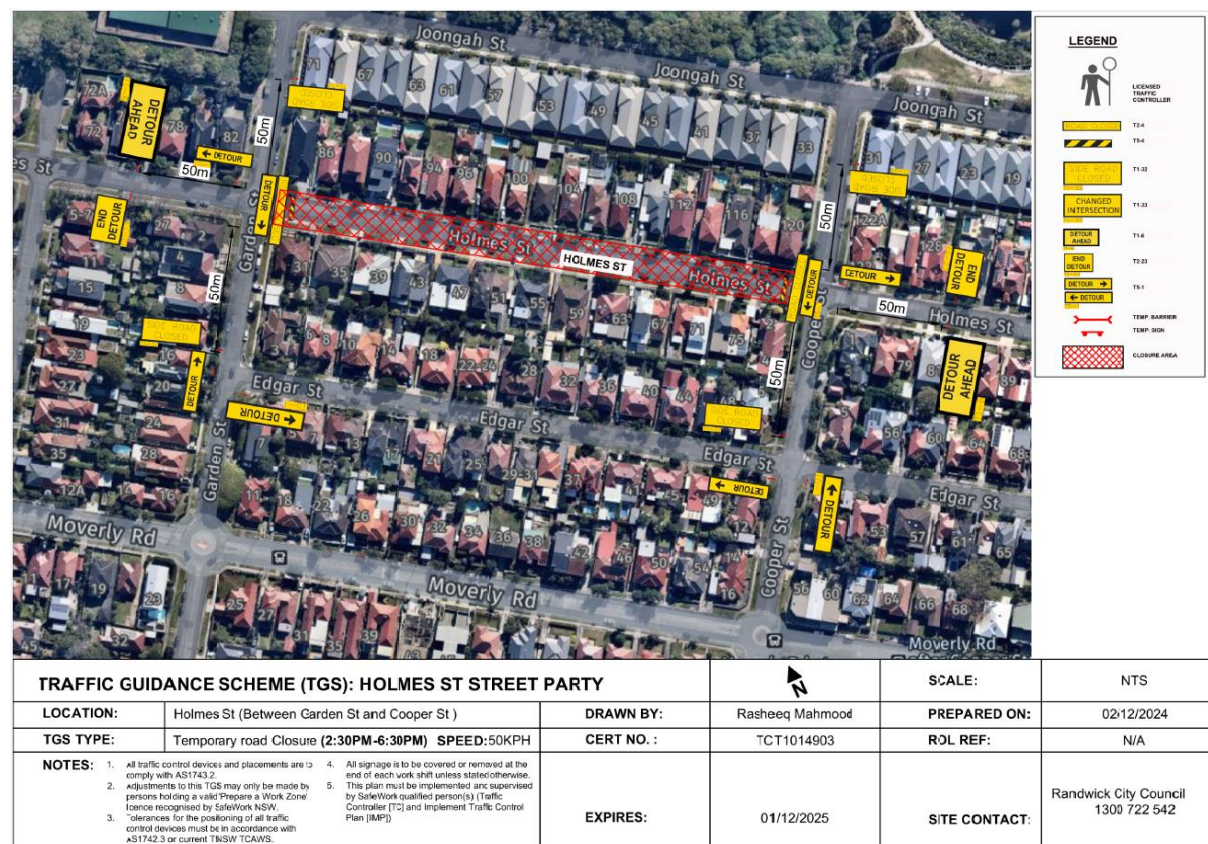
Figure 15: Holmes Street, Maroubra (M) Traffic Guidance Scheme
