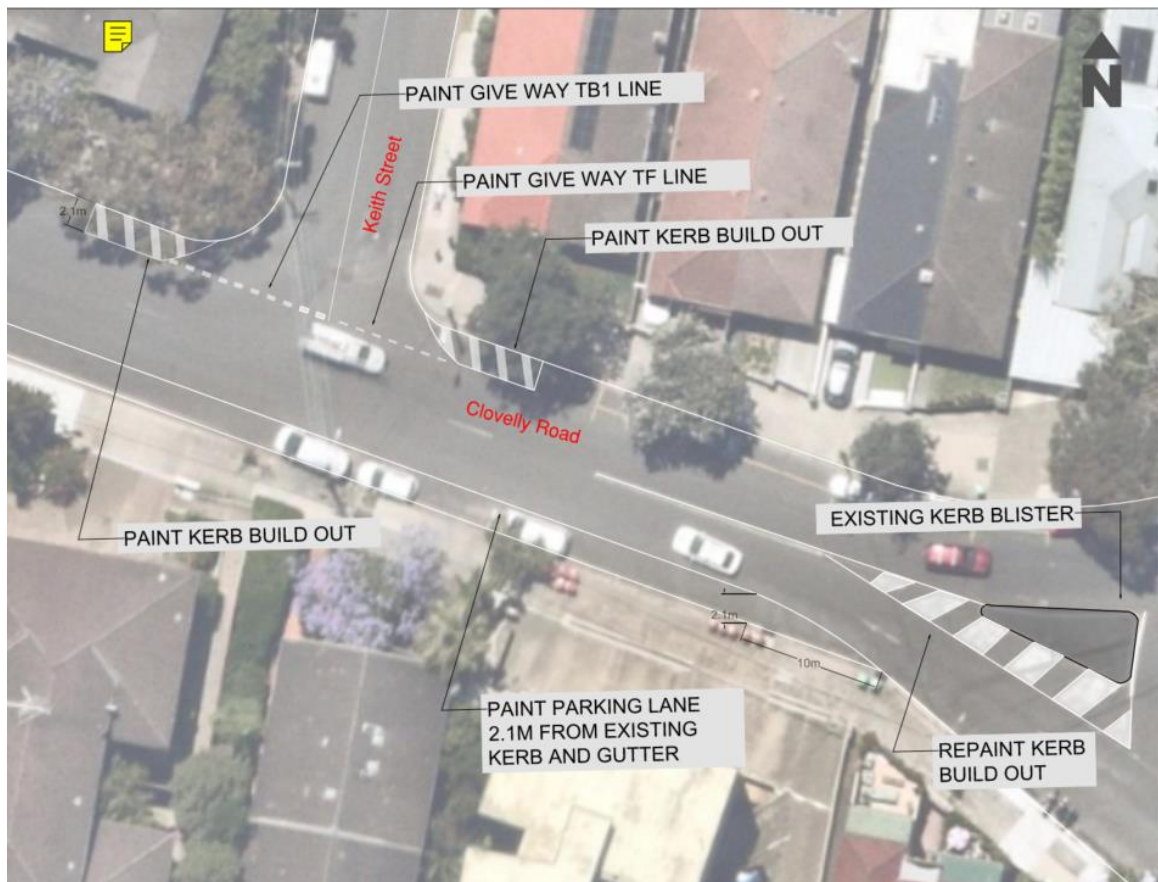
Fig:1 Concept Plan for Painted Chevron and bring forward the Give Way control
