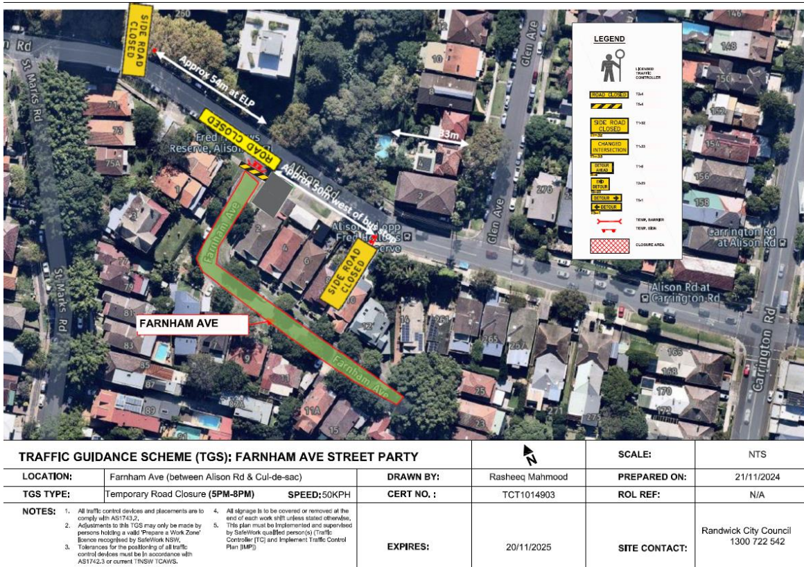
Figure 4: Farnham Avenue, Randwick (C) Traffic Guidance Scheme
