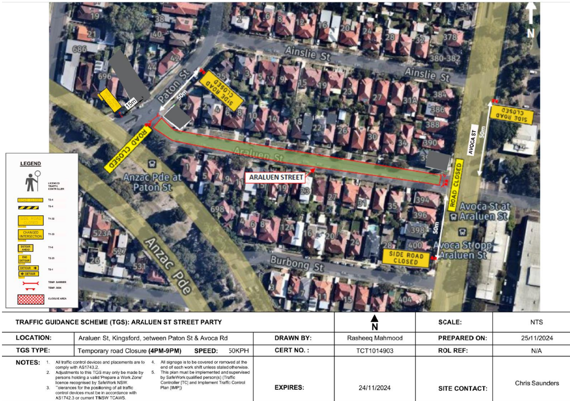
Figure 8: Araluen Street, Kingsford (H) Traffic Guidance Scheme
