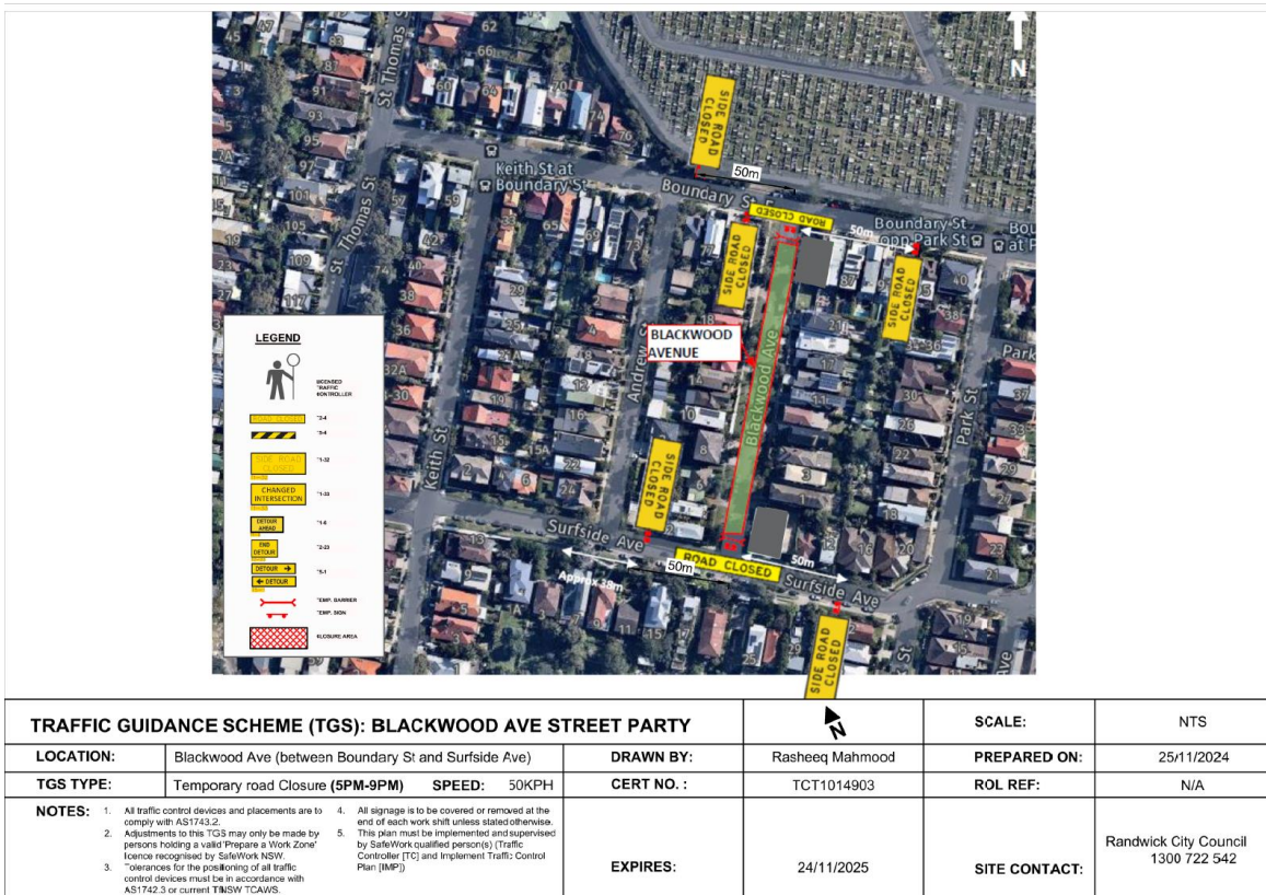
Figure 9: Blackwood Avenue, Clovelly (C) Traffic Guidance Scheme
