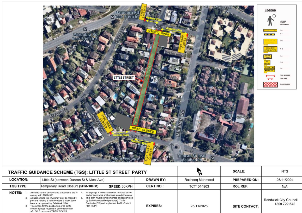
Figure 10: Little Street, Maroubra (M) Traffic Guidance Scheme
