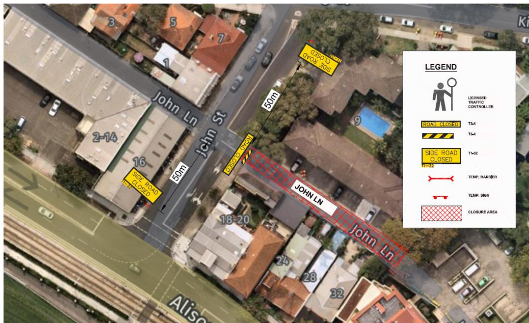
Figure 2: Aboud Avenue, Kingsford (H) Traffic Guidance Scheme
