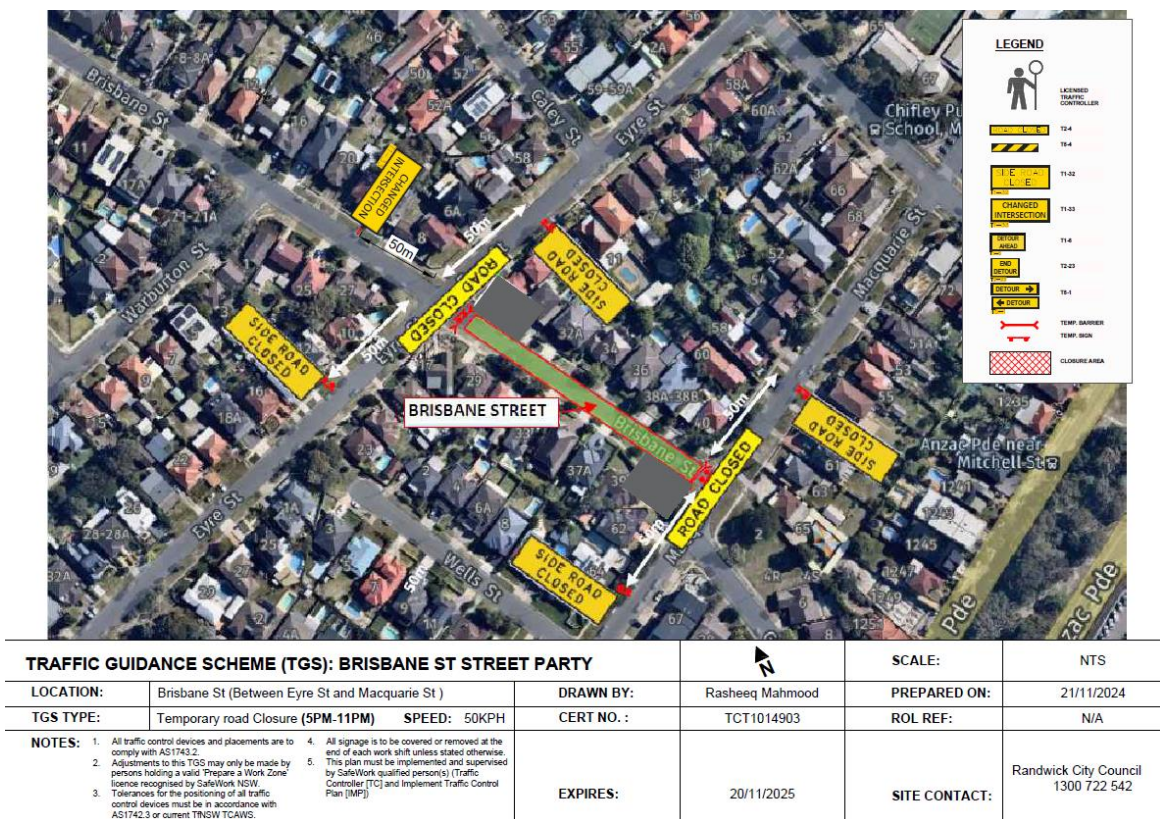
Figure 5: Brisbane Street, Chifley (M) Traffic Guidance Scheme
