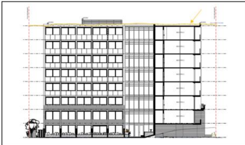
Figure 1: Section drawing with the height standard shown dotted in the architectural plans, highlight above in yellow for clarity.
