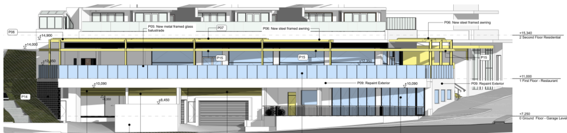
Figure 20: Northwest elevation showing the proposed awning structure (Source: Applicant)
