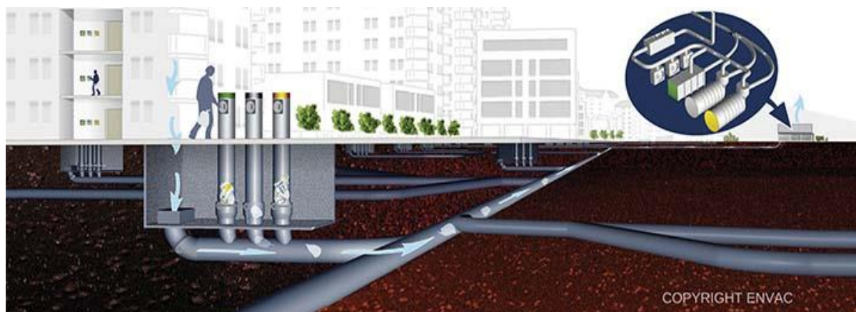
Figure 1: Centralised AWCS example
