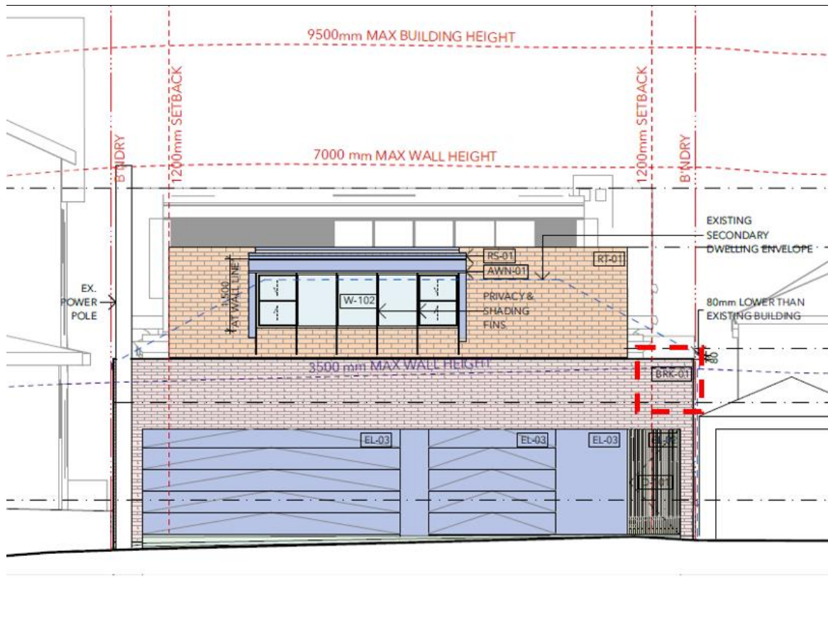
Figure 7 – Proposed modified laneway elevation showing the rear pedestrian entry. Note the section of wall dotted in red is required to be removed to match the adjoining garage (Condition 2f).
