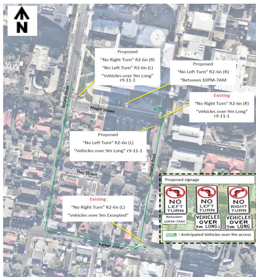
Fig 1: proposed turning restriction for vehicles over 89m long in Magill Street.
