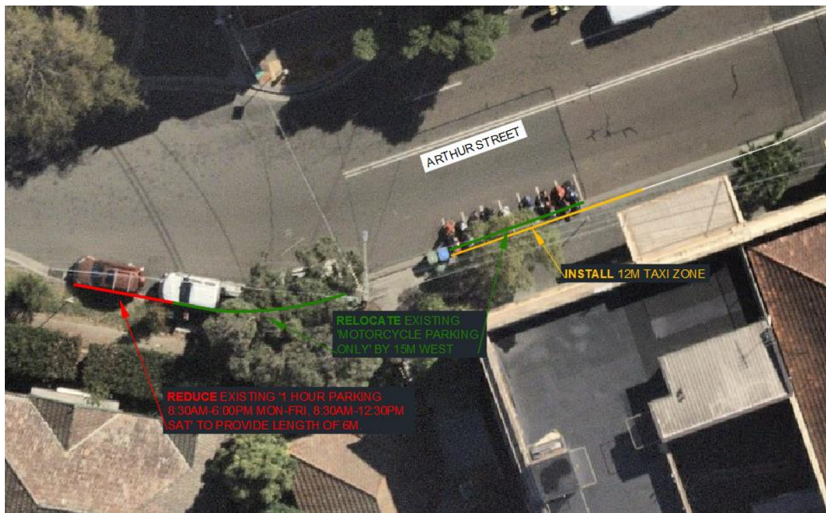
Figure 1: Arthur Street 12m Taxi Zone resulting in the relocation of the existing No Stopping Signage and the Motorcycle Parking Area.
