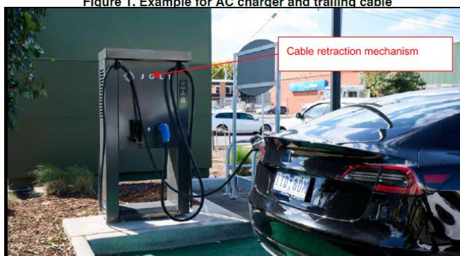
Figure 2. JOLT charging podium while in use. Highlighting cable retraction mechanism.
