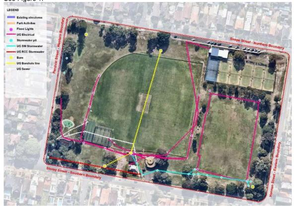
Figure 1 - Snape Park Underground Services Location (Bore water Line in Yellow)
