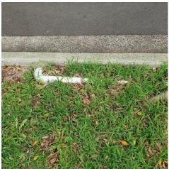
Photo 12. PVC pipe that has been crushed by the tree roots.
