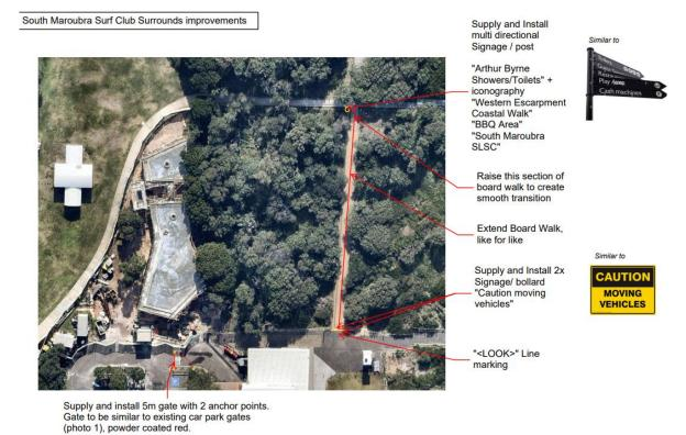
Figure 1 - Scope of Works Mark Up
