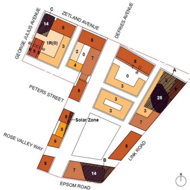
Figure 11: Extract from draft DCP – maximum number of above ground storeys (Source CoS draft DCP 2023)
