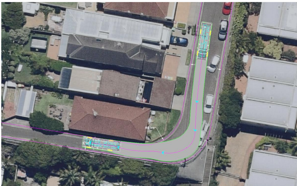
Figure 2 - Swept path - 8.8m service vehicle
