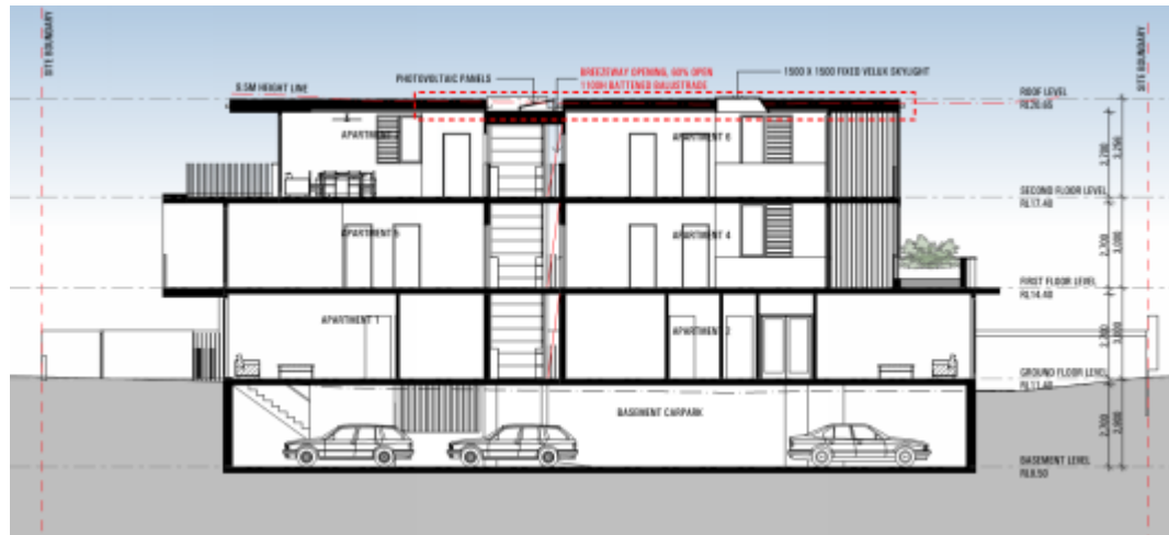
Figure 1: Section running through the building – red dashed lines showing non-compliant height section
