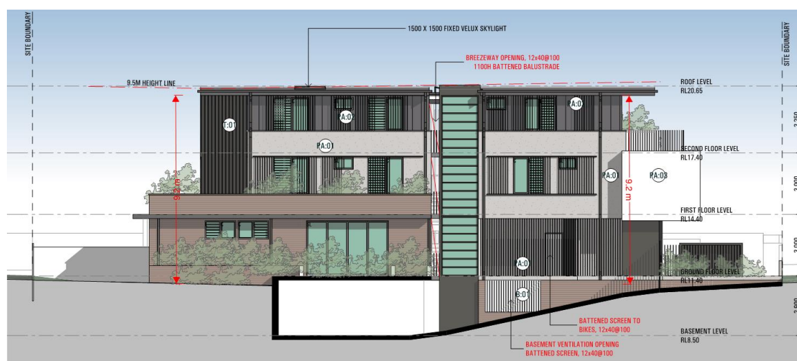
Figure 1 | Excerpt from Prescott Architects, East Elevation and Materials, A3101, Issue D dated 20 August 2019, showing the maximum external wall height of the building.
