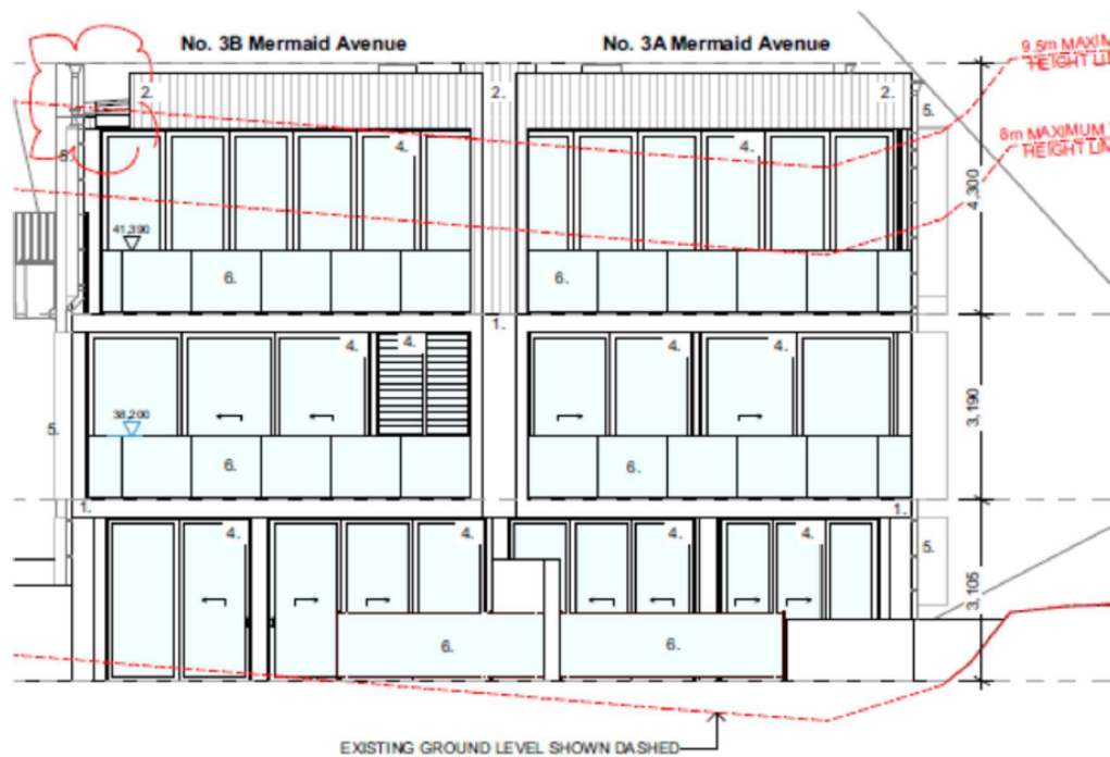
FIGURE 2: EXTRACT REAR ELEVATION SHOWING HEIGHT STANDARD
